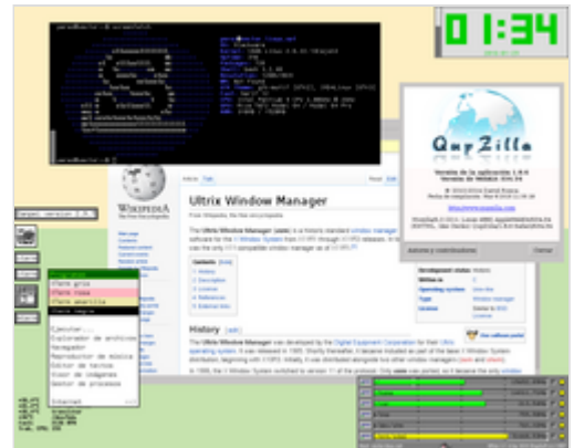
A screenshot of Ultrix Window Manager , which uses a stacking window manager. Note how the stacked windows overlap each other.
